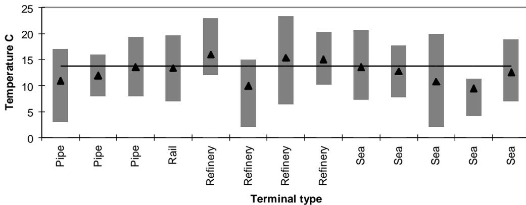
Fig 14 Operating Temperature Range for 13 terminals
