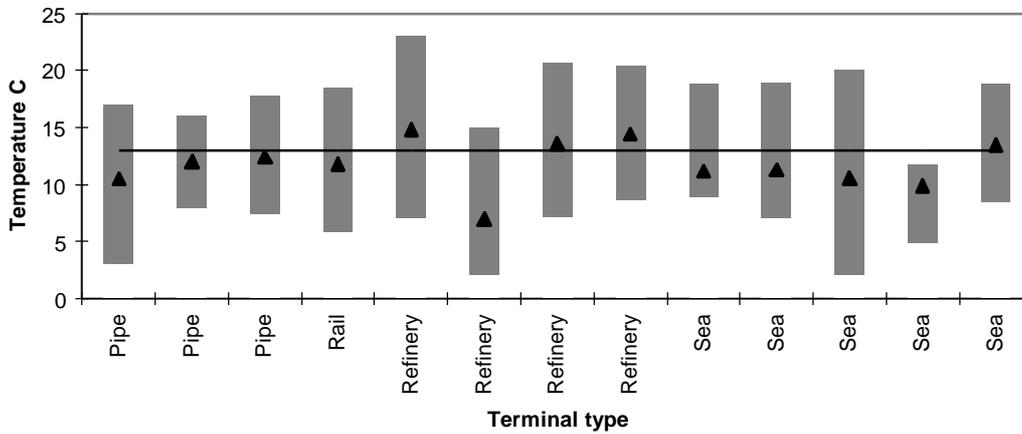
Fig 13 Operating Temperature Range for 13 terminals
