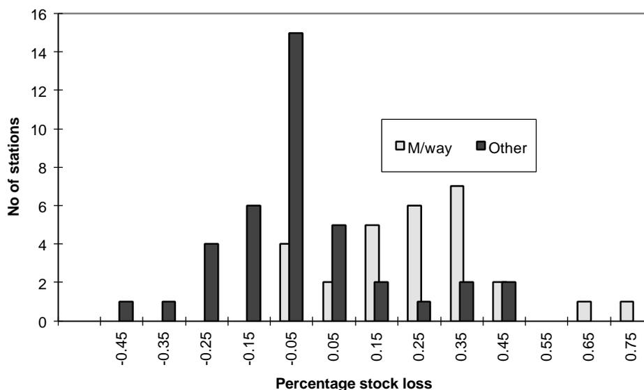
**Fig 2 PRA Survey of Diesel Stock Losses**
